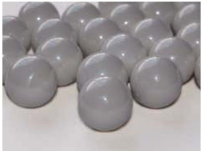
Grey Silicon Nitride Balls
